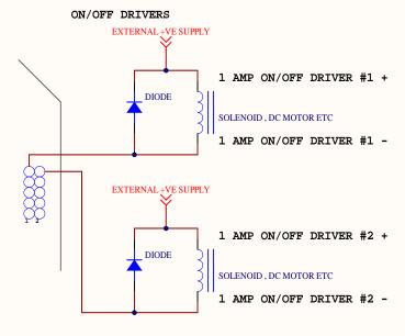
EXTERNAL SUPPLY VOLTAGE MUST BE LESS THAN SUPPLY TO EZ STEPPER
